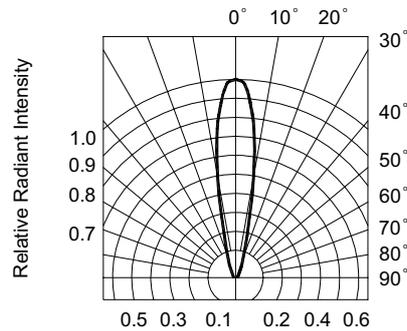
FIG.6 RADIATION DIAGRAM
