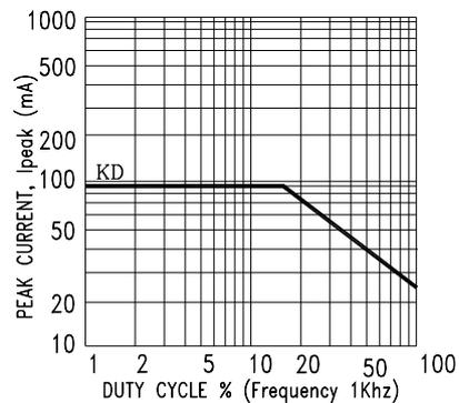
Fig5. Maximum Peak Current vs. Duty Cycle %
