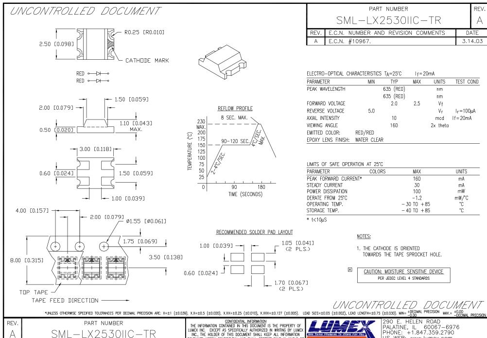
3.0mm x 2.5mm SURFACE MOUNT LED. BICOLOR. DUAL RED/RED CHIPS, WATER CLEAR LENS, TAPE AND REEL.
